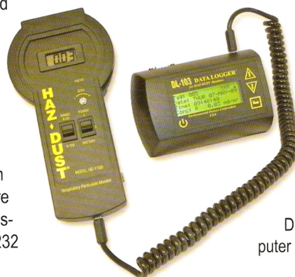
Measuring Oil Mist Particulate Concentration in machining application
