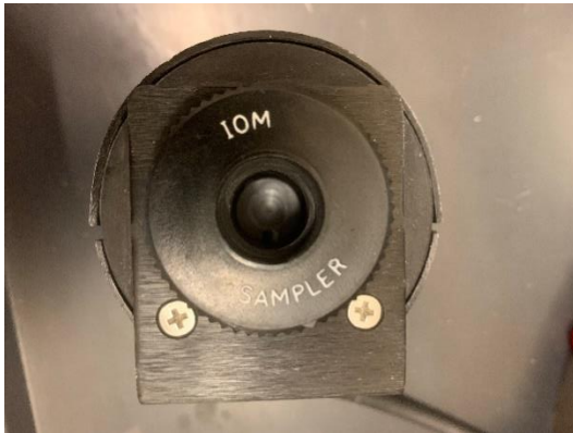
Photo 3. IOM-type HD-7204 Sampling Head.
