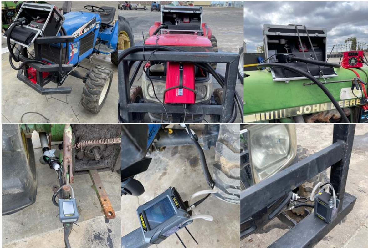
Figure 1. NOVA Plus gas emissions monitor (top), Haz-Dust HD-7204 PM monitor (bottom) setup on the diesel vehicles to be tested for emissions.
