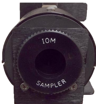
Figure 4: ISO Validated IOM for Inhalable
