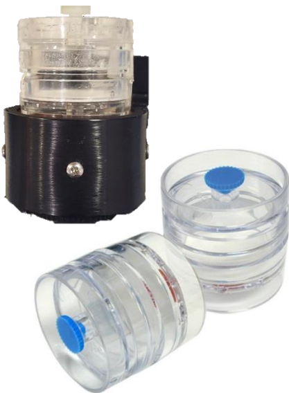
Figure 2: Accepts any ISO pre-weighed laboratory 37mm cassette.
