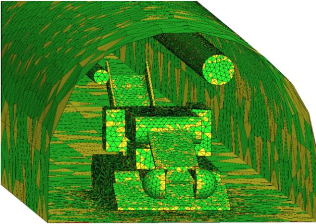
Fig. 8. Geometry and model meshing for the E-R auxiliary ventilation system.
