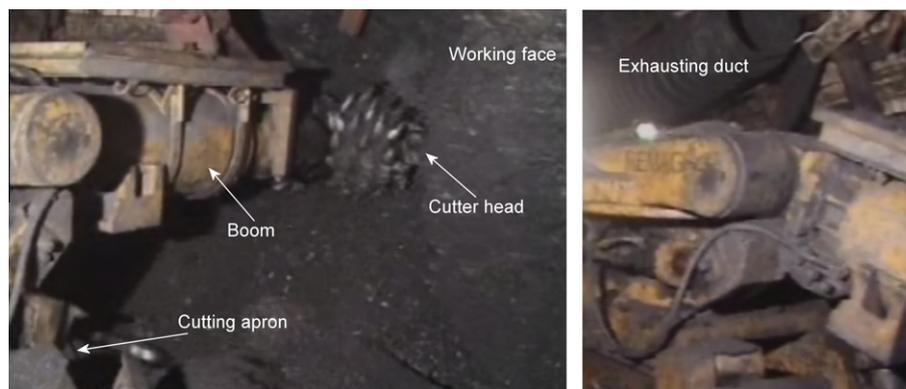
Fig. 2. AM50 roadheader driving the roadway in the coalbed.
