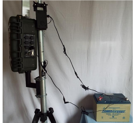
Figure 13. Connection from HAZ-SCANNER and Temperature Relative Humidity to Backup Battery
