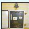
Low cost Filter Based PM-2.5 and PM-10 Air Sampler Dust-Sol DS-2.5 Portable Particulate Ambient Air Sampler
